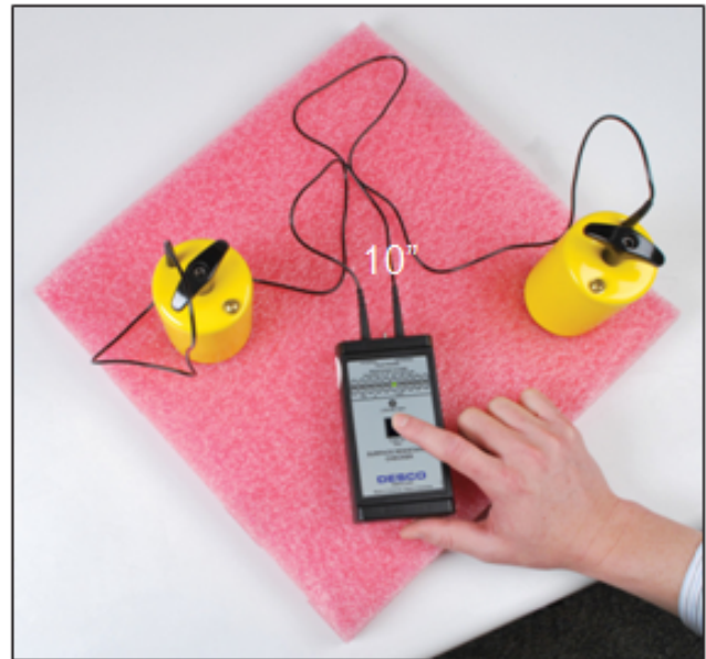
Figure 4. Using the test leads and two 5 pound electrodes to measure RTT
