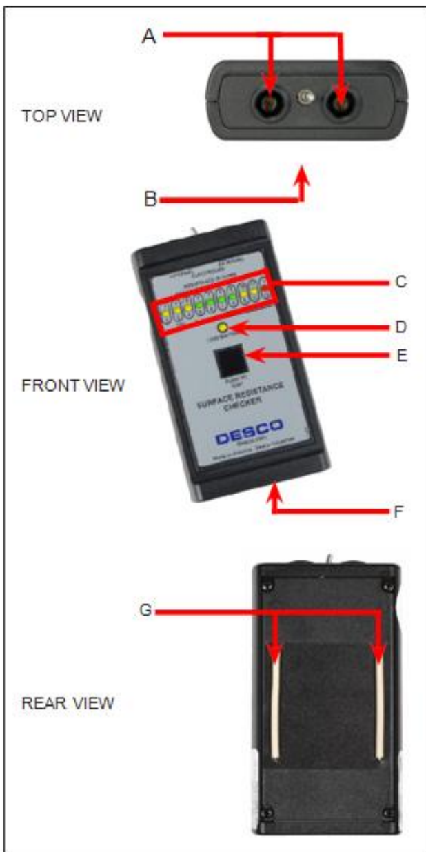
Figure 2. Surface Resistance Checker features and components
