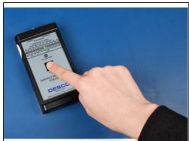
Figure 3. Using the internal parallel electrodes to measure surface resistance
